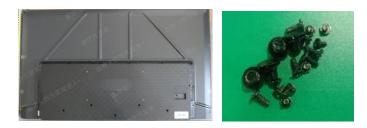
Once removed, this will expose the PCBs Units, which can now be easily removed with hand and screw driver, remove the WIFI module, key pad and IR.
